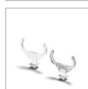
Lamp supports for TC-L lamps Height adjustable H: 31/34/37 mm Push-fit foot for cut-out ∅ 5.5 mm for wall thickness up to 1 mm Weight: 0.7/1.3/1.1 g, unit: 500 pcs.
