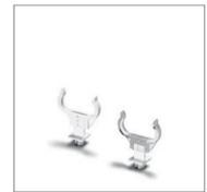
Lamp supports for TC-S, TC-SEL lamps Height adjustable H: 27.5/30.5/33.5 mm Push-fit foot for cut-out Ø 5.5 mm for wall thickness up to 1 mm
